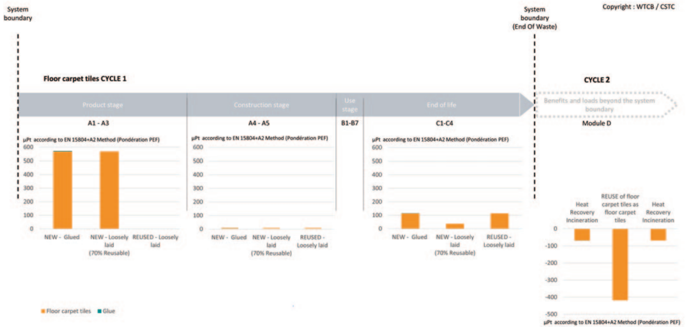
Figure 002: Comparing the environmental impact of three 1m 2 floor coverings: reused loose-lay carpet tiles; new carpet tiles with adhesive; and new loose-lay carpet tiles.
