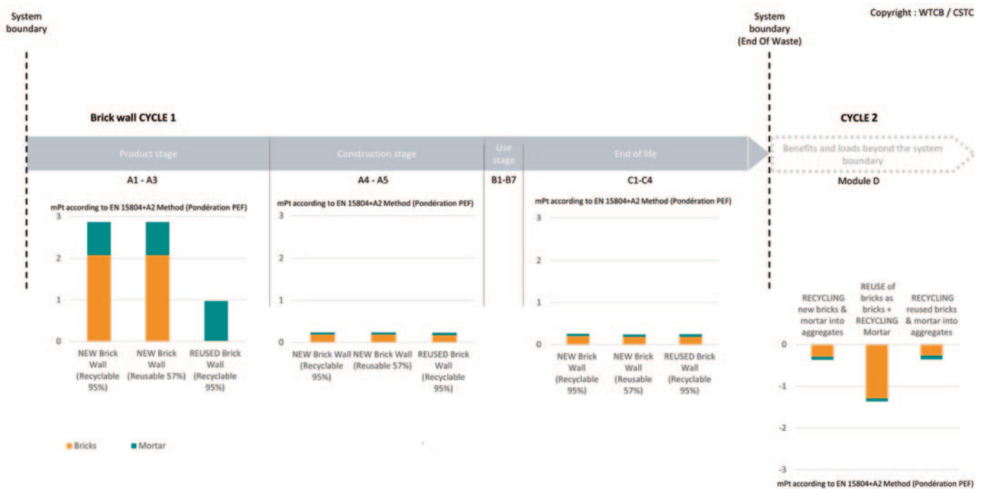
Figure 001: Comparing the environmental impact of three 1m 2 walls built using new recyclable bricks, new reusable bricks and reused bricks
