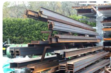
Storage of beams by profile and shape © Opalis (Sarl Perrin)
