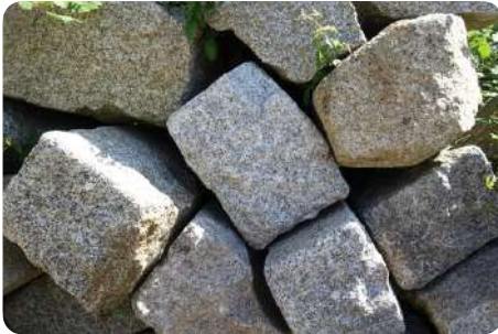
Reclaimed kerbs in grey granite
