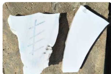
"Porous" glaze vs glaze in good condition
