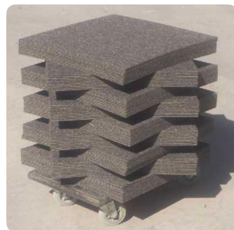
Movement of tiles using trolleys. The staggered arrangement facilitates handling.
