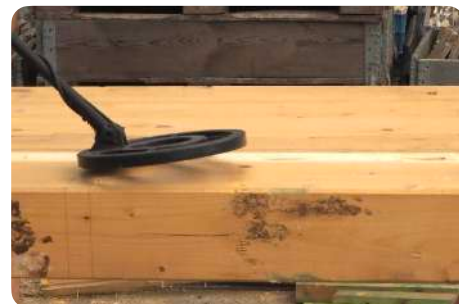
Metal detector inspection
