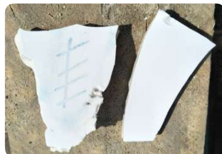
"Porous" glaze vs glaze in good condition
