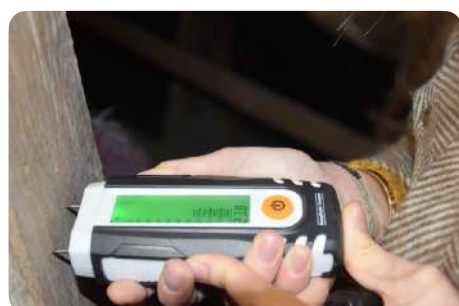
Wood moisture measurement using a moisture meter © Romane Lavoine
