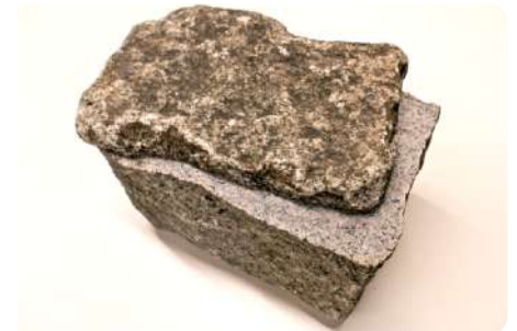
Sawing of the upper part of the stone sett
