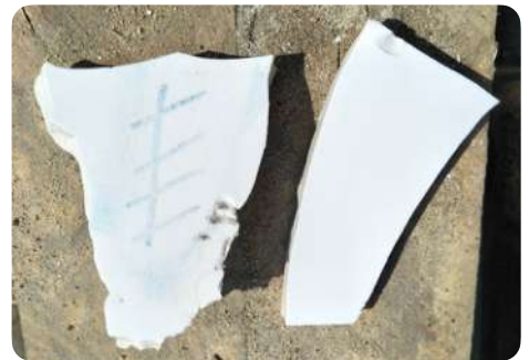
'Porous' glaze (left) vs glaze in good condition (right)
