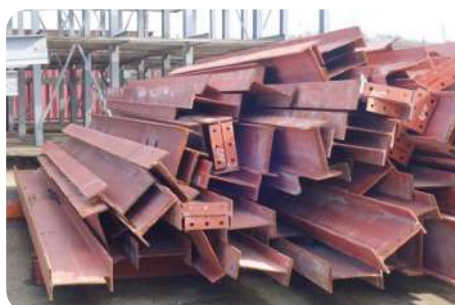
Reclaimed IPE beams, with anti-corrosion protection treatment. © Opalis (Omgekeerd Bouwen)
