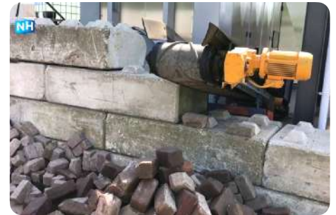
Automated cleaning and packaging process for reclaimed clay pavers. © NH Nieuws, 2018 ( https://www.youtube.com/watch?v=lmeWIMkRwoU )
