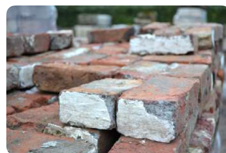
Traces of paint and slight remains of mortar
