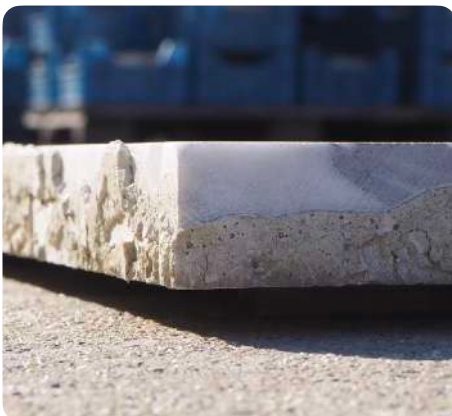
Residue on the side of a reclaimed marble tile
