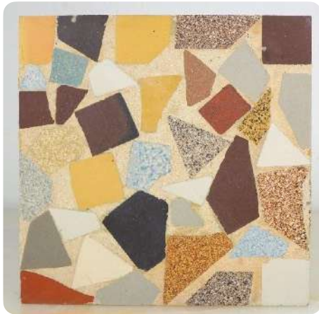
Terrazzo tile whose aggregate is made up of offcuts of porcelain stoneware tiles
