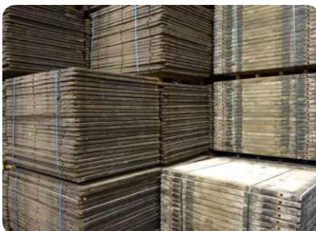
Reclaimed timber formwork steenschotten panels
