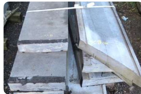
Sealant and tar residues © auctelia
