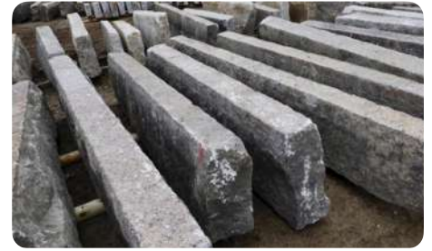
Kerbs in old natural stone (<19th century) - manually cut - thick and irregular. © stonecurators.com
