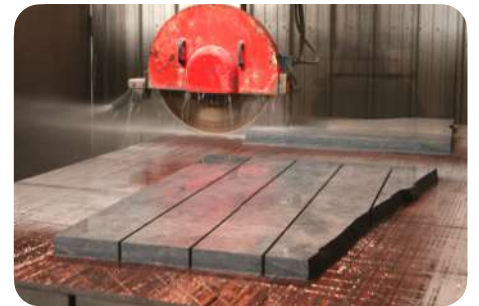
Cutting stone elements
