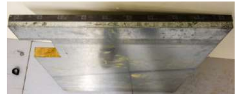
Incomplete covering, uncoated, based on chipboard, encapsulated in a galvanised steel sheet. Half of the edge is provided with a self-extinguishing PVC strip.
