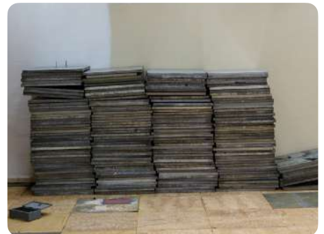
Deformed or non-compliant coverings, not recovered.
