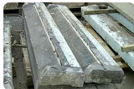
Traces of remaining mortar © valleyreclamation.co.uk
