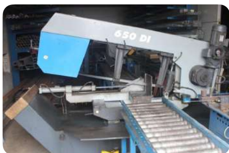
Installation for cutting beams © Opalis (Wolter Bouwmaterialen)
