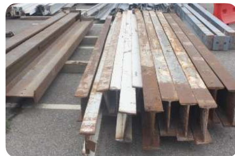
Storage of recovered beams on wooden supports © Opalis (Premys Ferrari)
