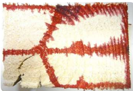
Red colour revealing an absence of treatment. © expert-bois.fr
