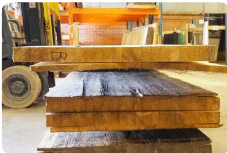
Splitter glued laminated timber (sawn lengthwise)
