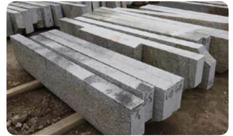
Natural stone kerbs later in the early 20th century - made using power tools - uniform and precise appearance. © stonecurators.com
