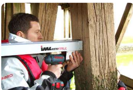
Hardness test using a resistograph © qsb.fr
