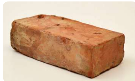
Beersesteen-type extruded reclaimed brick (BE)
