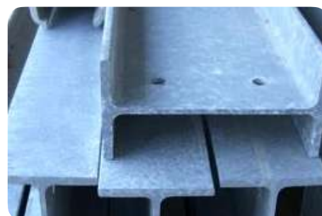
Galvanised steel beams © lecoindupro
