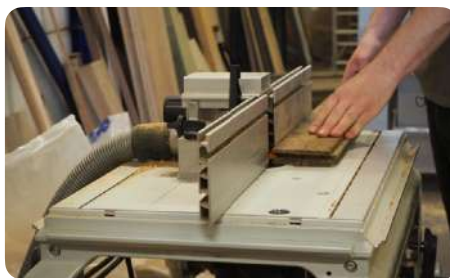
Re-machining of tongue and groove
