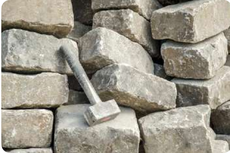
Reclaimed sandstone kerbs
