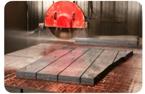
Cutting stone elements
