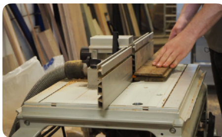
Re-machining of tongue and groove
