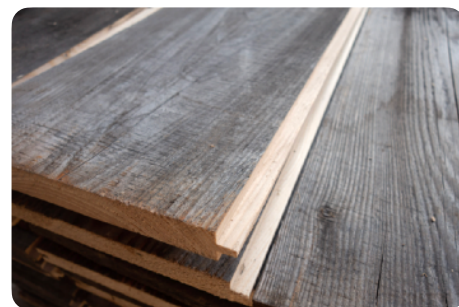
Machining of boards to obtain a tongue/groove assembly profile
