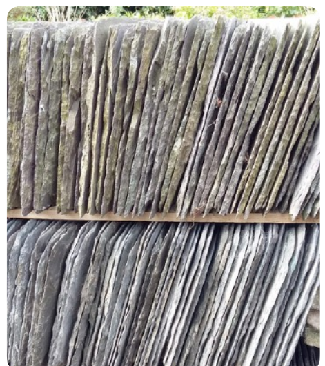
Storage of reclaimed slates © hastingswhite.co.uk
