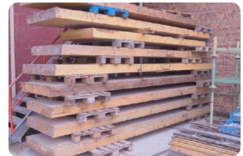
Storage of reclaimed glulam beams
