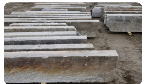
Kerbs in old natural stone (19th - 20th century) - the upper face is sawn and the other faces cut manually - more regular shape. © stonecurators.com
