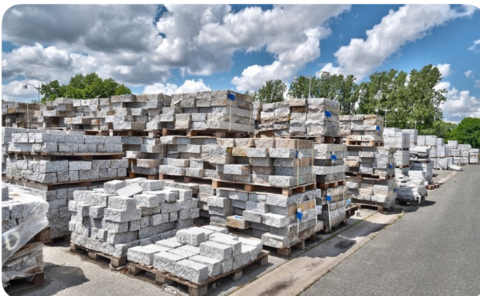
Paris paving depot, Bonneuil-sur-Marne. Stock of cobblestones and stone kerbs ready to be sorted, cleaned and reused in sites in the city of Paris (FR) © Ville de Paris, Florence Morisson.
